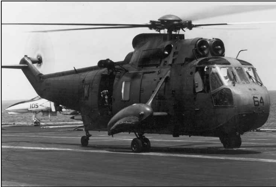
Left: The Sikorsky HH-3A, a modification of the sub-hunting SH-3A, was reconfigured with upgraded engines and armor surrounding critical components and crew stations, plus extended-range fuel cells. Eleven CSAR Sea Kings were finally made available for operations in Vietnam. Big Mother 64 is shown on the flight deck of USS Coral Sea (CVA-43) toward the end of the War in Vietnam, 26 Sep '73. Below: An HH-3A is shown on alert on board a guided missile frigate, ready to launch within five minutes of being called. It took a steady hand to maneuver the large Sea King onto the tiny flight deck with minimum clearance ahead of and behind the helo. Despite this, landing incidents were relatively few.
