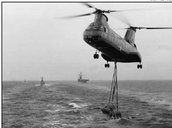
In addition to CSAR, HC-7's mission included vertical replenishment responsibility for 7th Fleet units. Techniques of the mission were transplanted from HC-4 at Lakehurst by LCDR Joe Gardner. HC-7's vertrep capability was later transferred to HC-3 at NAS Imperial Beach. An HC-3 UH-46A is shown with two pallets of Mk 82 bombs bound for the Essex-class carrier on the horizon.
