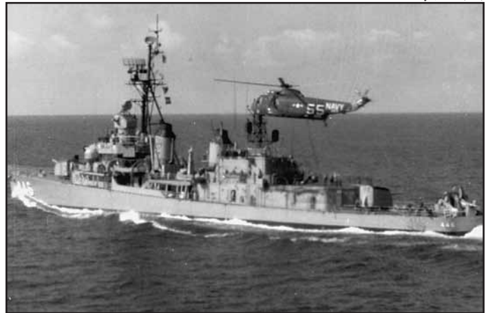
Helo inflight refueling from a destroyer extended the range of the Sikorsky SH-3A, thus making it an ideal search and rescue vehicle. An HS-6 Sea King hoists a refueling hose from the drone helo deck of USS Radford (DD-446) to fill its tanks with as much as four hours of fuel.
