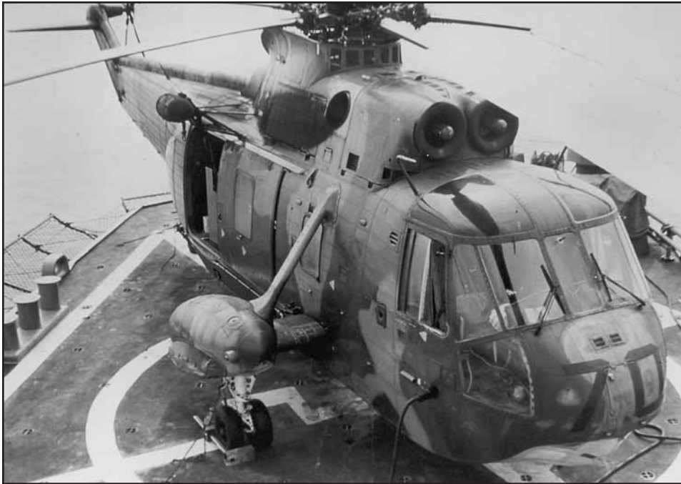
Left: Big Mother 70, an HS-2 SH-3A, sits on Alert 5 on the fantail of USS Mahan (DLG-11). The landing area on SAR ships was tight—only a few feet clearance existed between the tailwheel and the deck edge; likewise between the main rotor and the aft missile launcher. Below: Bennington (CVS-20), with HS-8 embarked, was one of four ASW carriers in the Tonkin Gulf that carried SAR H-3s. The others were Hornet (CVS-12) with HS-2, Kearsarge (CVS-33) with HS-6 and Yorktown (CVS-10) with HS-4.
